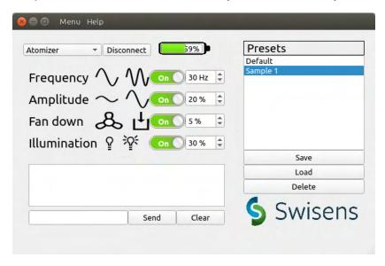
The combo box in the upper left corner lists connected Atomizer devices. A connection can be opened using the button adjacent. Next to the button is a display of the remaining Atomizer battery charge.
